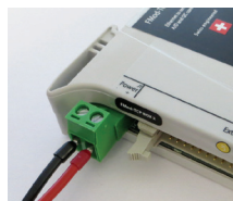
Power connector 12 – 33 VDC (Female connector PTR AKZ950 is provided with the device)
